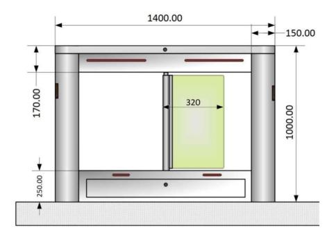
Swing turnstile has standard electrical interface which can be connected with ID cards, IC cards, magnetic cards, barcode cards etc. The arm will open automatically when turnstile received relay signal.
